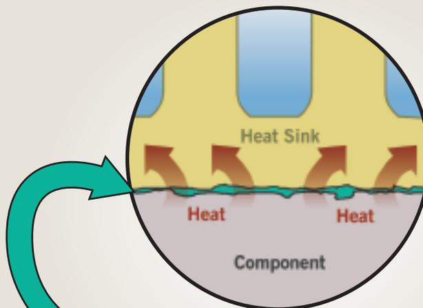
By filling in surface imperfections of the heat sink and component, the compound effectively transfers heat into the heat sink.
