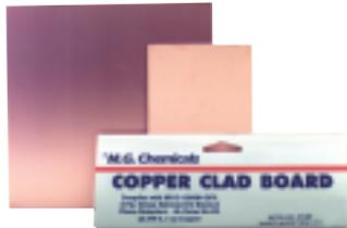
A 1/16", 1/32", 1/64" laminate with 1 ounce copper. This flame retardant laminate is made of continuous woven glass cloth impregnated with epoxy resin. Developed specifically for the circuit processing industries' requirements. Provides ultraviolet blocking and fluorescence when using automated optical inspection (AOI).
