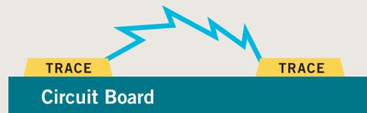
Arcing occurs when voltage jumps from one surface to another due to the close proximity of parallel currents. The result is a board malfunction or damaged components. It may occur on any circuitboard without a coating.
